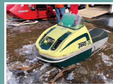
The Burdick family's 1971 Eskimo RT/2. The sled is all original and is powered by a 38 horsepower 436cc Sachs engine. Photo/John Lumnah.
