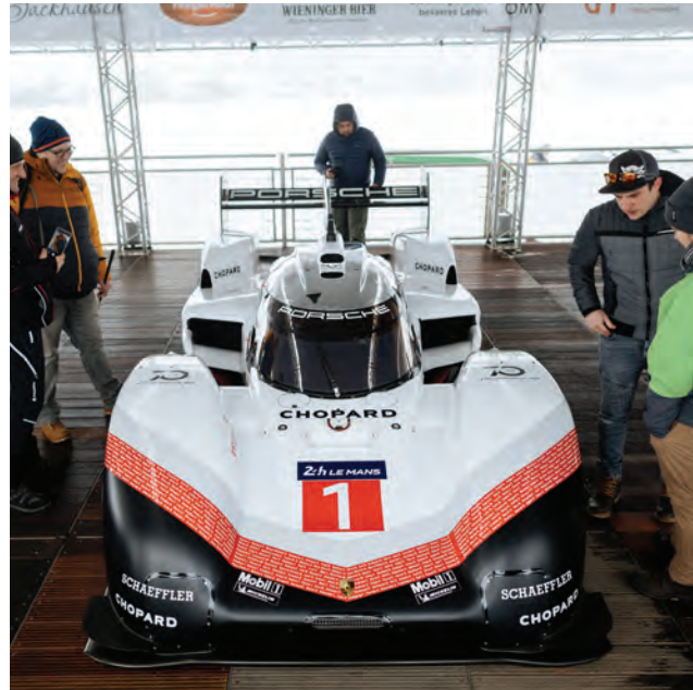
The Porsche 919 Hybrid is amazing. During braking, a generator at the front axle converts the car's kinetic energy into electrical energy. In the split exhaust system, one turbine drives the turbocharger while another converts surplus energy into electrical energy. Photo/Porsche AG
